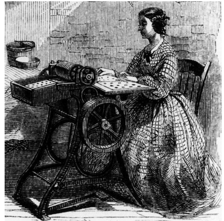
Bemrose-style Perforating Machine (ca. 1861)
